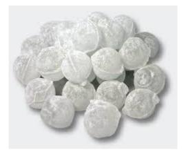
2) Ion exchange with the help of resins for adsorption of iron and calcium
