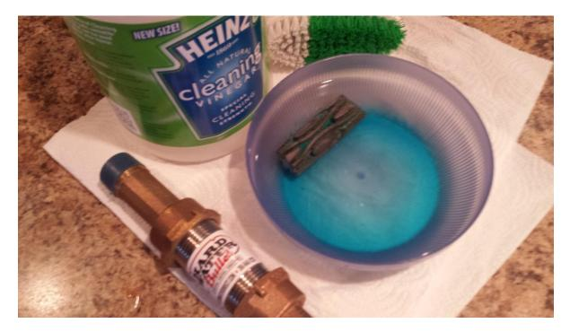
Cleaning the conditioners core every few months (Possibly more often if you have high iron in your water) will ensure that the conditioner will work at it's peak performance. It's important to install the core with the beveled end on the water inlet end of the housing, This is because a venturi effect is created when the water enters the cores beveled end .
